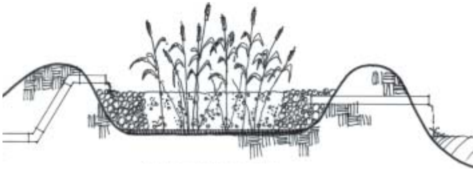
From top: A planted rock filter is ideal for alternately wet and dry conditions, provides more planting flexibility, and is effective for stormwater as well as wastewater. A freewater surface constructed wetland is always saturated, allowing for fish and wetland habitat, whereas the subsurface-flow wetland is dry at the surface and can be walked on. The planted evapotranspiration system is by design unsaturated or dry and lined and is chosen for environmentally sensitive sites where no wastewater can be discharged.
